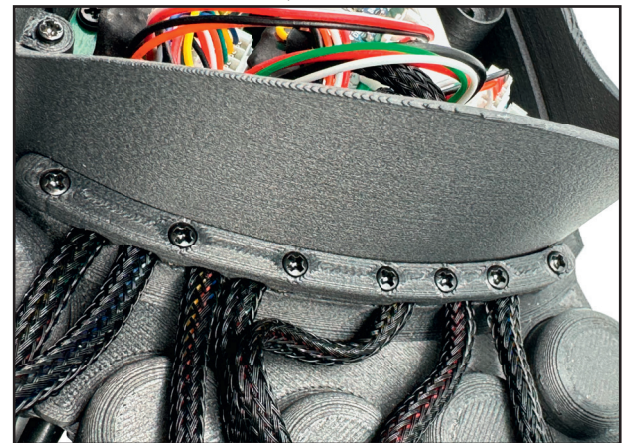
Figure 4-73: Final result of installed base rise and key strain relief.
