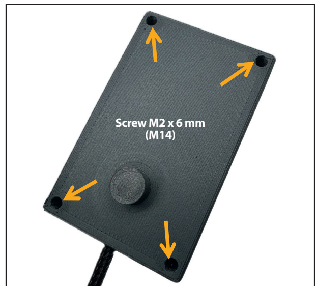
Figure 4-41: Inserting the screws into the display housing.
