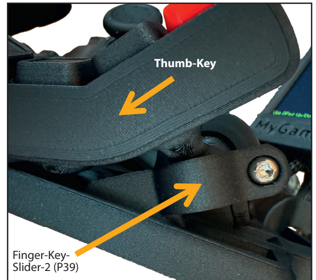
Figure 4-61: Thumb key element.
