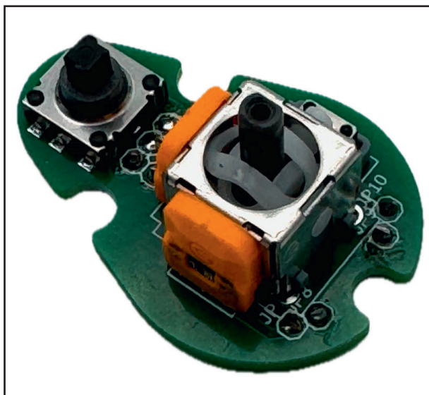
Figure 4-32: Placement of components on the Thumb-Stick-PCB.
