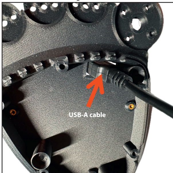
Figure 4-64: Inserting the USB-A connector through the hole.
